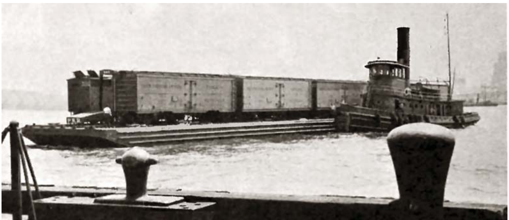
Two illustrations from the 1949 pamphlet Pennsylvania Railroad Harbor Facilities: Port of New York (Pennsylvania Railroad Company 1949) were captioned as follows: (TOP) "Three units of Pennsylvania's fleet of floating equipment—a covered and a refrigerated lighter being handled in tandem by a tug up Hudson River." (BOTTOM) "One of Pennsylvania's fleet of 70 modern steel carfloats with loaded cars aboard, being transported across the Hudson River."
