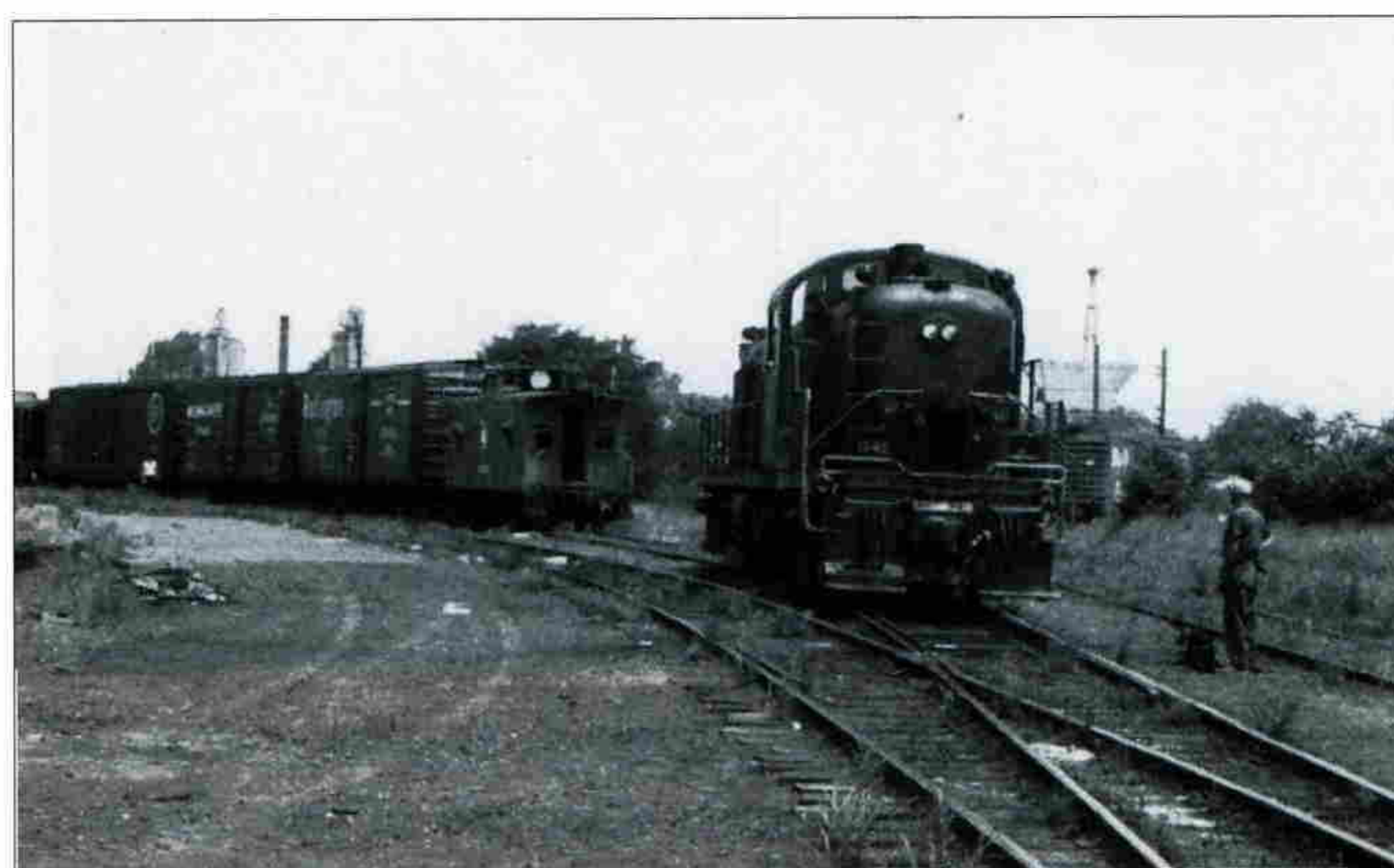
During the mid 1960s, Red Bank-based local freight QV-1 usually was powered by an Alco RS3 and had a wood caboose as shown in this July 1966 scene in Matawan yard.
